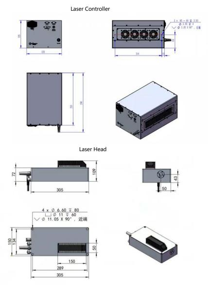
The controller and the output head are connected by a non-detachable optical fiber, the length of the optical fiber is > 1.5 meters
