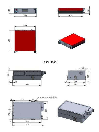
The controller and output head are connected by a non-detachable cable, the cable length is > 7 meters (customizable)
