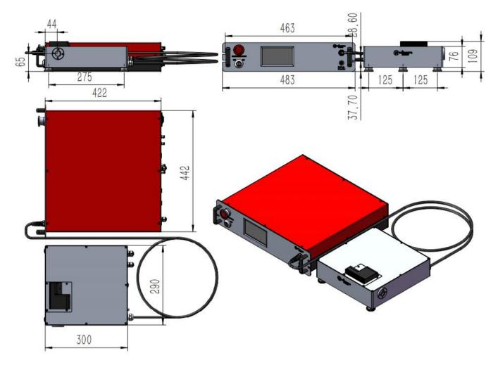
Non-dismantle fiber length  $\geq$ 2m between controller and laser head
