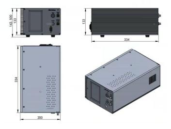
Laser Controller: includes power supply, current source and temperature control
